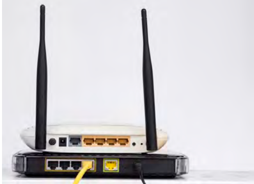
Router, rear side, view of the RJ connections and some buttons
