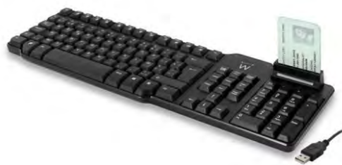
Keypad that contains a card reader. The card contains a chip that stores our digital ID
